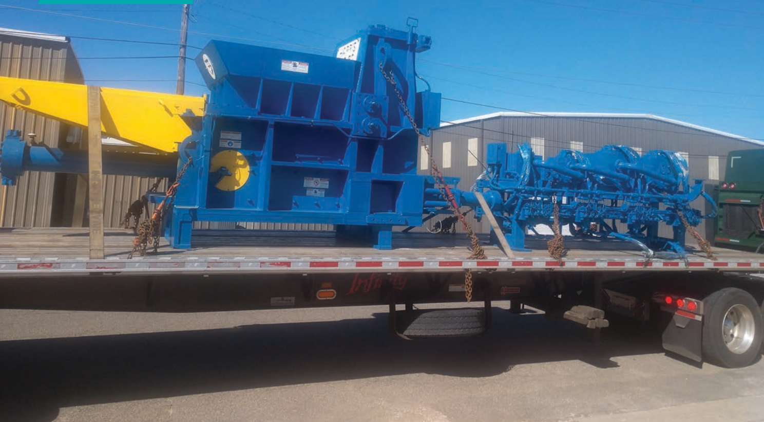
Harris Equipment's recycling products such as this cardboard bailer require tapping extremely durable wear plate liners made from Hardox 450 steel (45 HRC). (All images provided by Harris Equipment)
